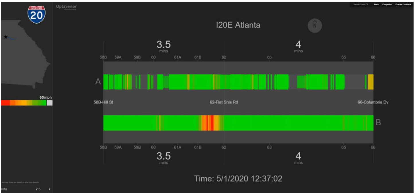
Screen shot taken from OptaSense Traffic Monitoring Solution indicating average traffic speed and journey times between distance points.
